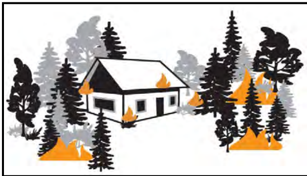
Figure 38 – Dense and overgrown vegetation poses a hazard due to continuous continuity that carries to the home.
