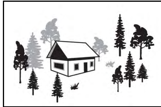
Figure 27 - Example of a well mitigated lot that is not clear cut but has adequate spacing between trees and the home.
