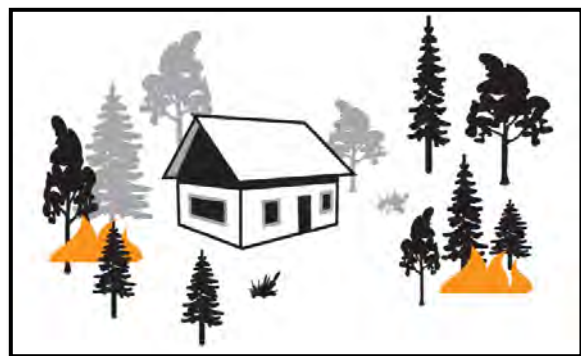
Figure 39 – Proper fuels management limits fire spread continuity and reduces the fire spread to the home.
